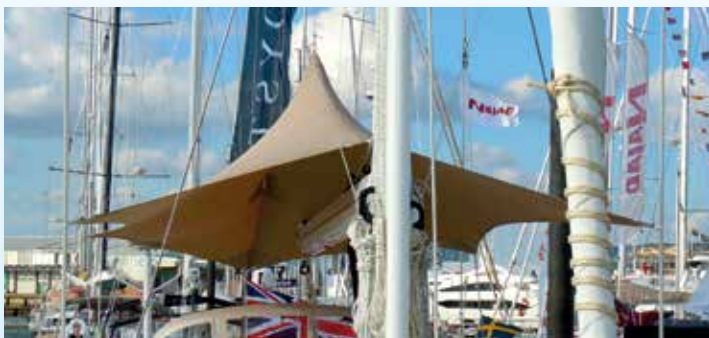
2. High central peak that is hoisted with the passarelle halyard or topping lift.
