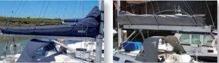
For the cruiser/racing customer you can upgrade the cover to have roll away clips added, this will allow you to easily detach or pull the lazyjacks forward and roll the cover sides away and clip them against the boom. This option cuts down on the windage on the cover sides and also allows better viewing of the mainsail sail shape.
