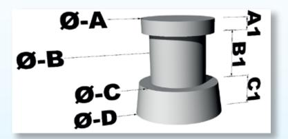
The above measurements are required for each winch cover that is needed. The colour will also need to be supplied along with the height of any plinths to which individual winches are fitted.
