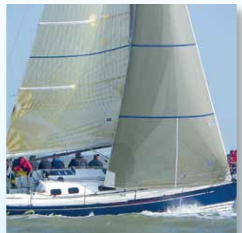
An X332 using a Membrane mainsail and Tri Radial headsail
