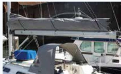
For the cruiser/racing customer you can upgrade the cover to have roll away clips added, this will allow you to easily detach or pull the lazyjacks forward and roll the cover sides away and clip them against the boom. This option cuts down on the windage on the cover sides and also allows better viewing of the mainsail sail shape.
